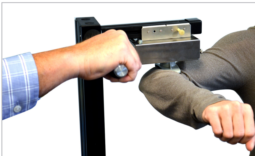
Example setup for Middle Deltoid test
