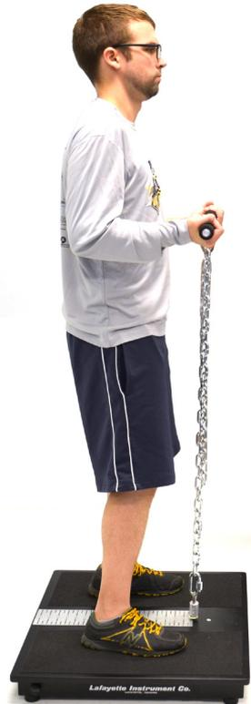
**Test Position for the Isometric Arm Strength**
