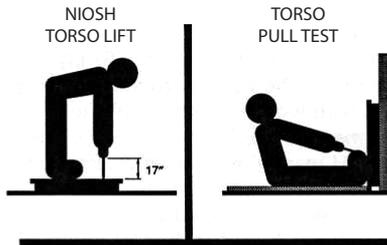
**The NIOSH (1977) Torso Lift Test and the Torso Pull Test
